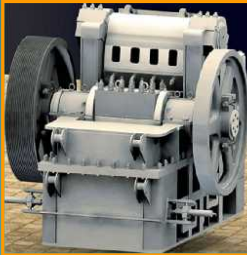
Jaw crusher with a simple swing of the cheek
