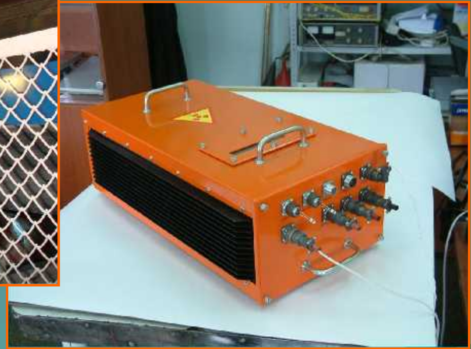
Ore Control Station (RCS-CM)
